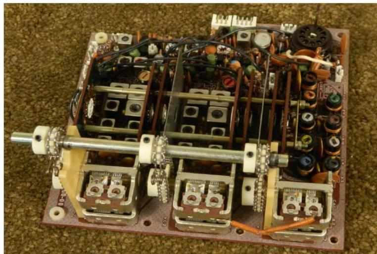
This is the RF board assembly as removed from the radio. It has only been cleaned by the use of compressed air to remove the loose dirt and dust.
