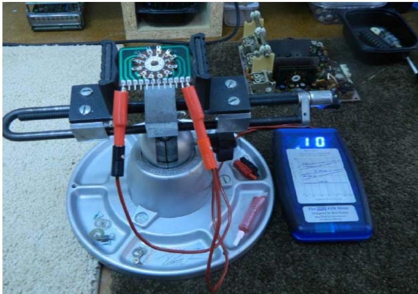
Each contact is checked for high resistance after cleaning. I am using here the Blue ESR meter which will measure quite low resistances. The reading here is .1 ohm. As you get closer to the other probe, the resistances will decrease as it is reading the resistance of the traces on the board. I also check physically for any looseness of the contact on the board. These contacts are originally held in place with rivets and they sometimes loosen.
