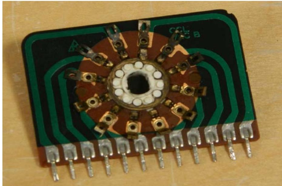
This is the first bandswitch wafer as removed from the RF board. You can see the buildup on the switch contacts and rotary contacts. This is not the worst I have seen by any means.
