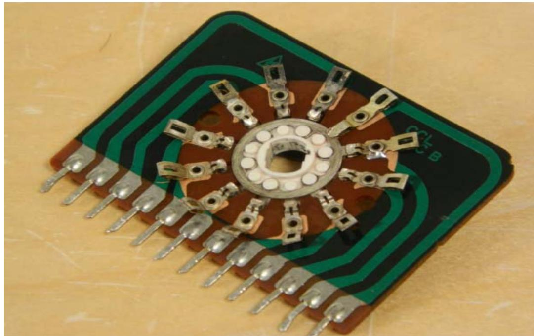
This is the same wafer after polishing to remove the dirt and tarnish on the contacts. I am now using a product made for polishing silver. It is called Wright's Silver Cream and works quite well. I use a discarded soft toothbrush to accomplish the cleaning/polishing and then rinse with tap water. The final rinse of the wafer is done with distilled water. The wafer is then carefully dried and blown out with canned air.
