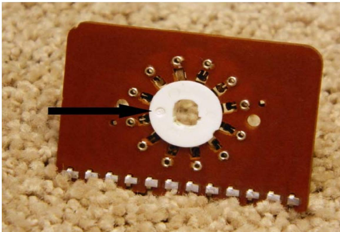
The rotary section of the switch must be properly aligned prior to installation so that each section will align properly with the switch shaft during reassembly. On the backside of the wafer are some marks that will be used for alignment. **VERY IMPORTANT!** Rotate the white collar of the switch so that the small recessed dot is at the nine o'clock position. When reassembling the switch, these will represent the 30 meter position on the bandswitch dial.
