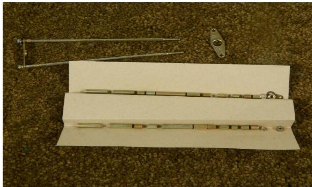
These are the through screws and spacers as removed from the switch assembly.
