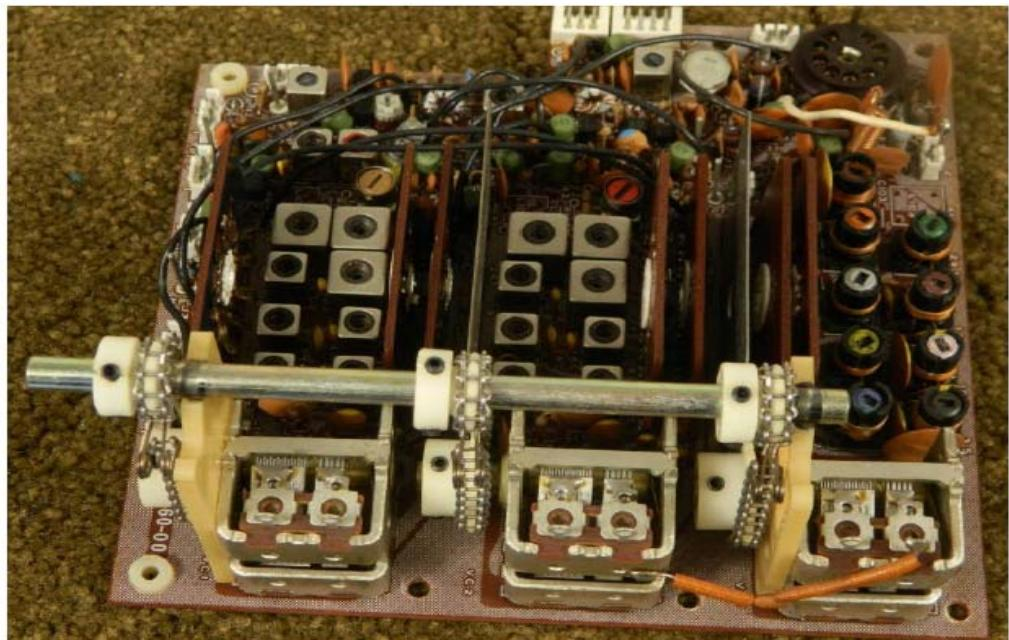
This is the same switch with the through screws and spacers removed. They are kept in order so that they may be replaced correctly.
