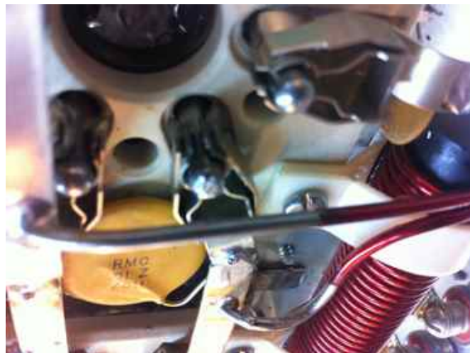
Tube replaced – filament pin nice and tight
