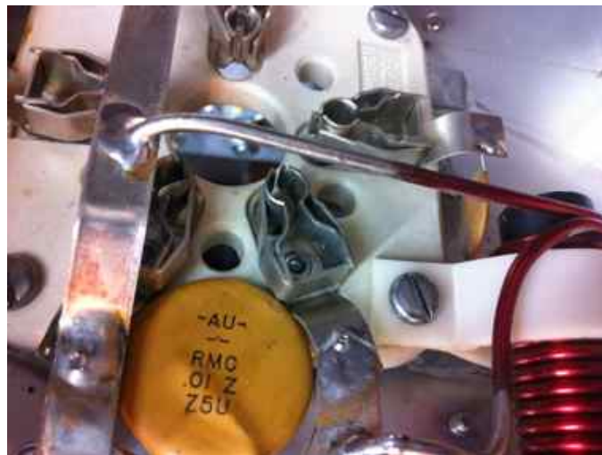
The loose tube socket pin – compare the clip closure to the others
