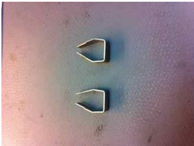
The replacement clip (top) compared to the loose clip
