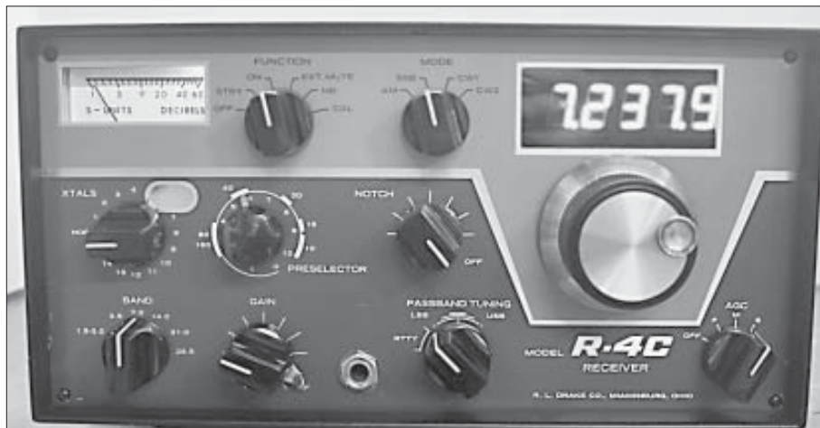
Figure 1: This classic Drake R-4C receiver has been upgraded with a modern digital display.
